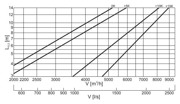
Max temperature difference for heating:  $\Delta t \leq$  15 K.
