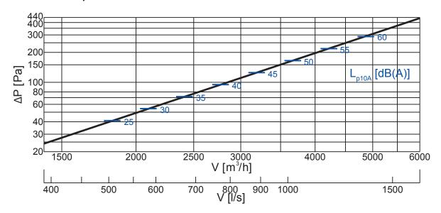
In the above graph, the sound pressure levels in dB(A) are indicated for a reference room with 10  $\rm m^2$  Sabine room absorption, equivalent to 4 dB room attenuation.
