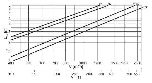
Max temperature difference for heating:  $\Delta t \leq$  15 K.
