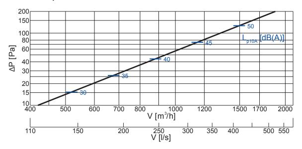
In the above graph, the sound pressure levels in dB(A) are indicated for a reference room with 10  $\rm m^2$  Sabine room absorption, equivalent to 4 dB room attenuation.
