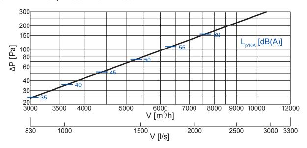
In the above graph, the sound levels pressure in dB(A) are indicated for a reference room with 10  $\rm m^2$  Sabine room absorption, equivalent to 4 dB room attenuation.
